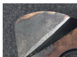
Flank and Rake wear after 45 min
