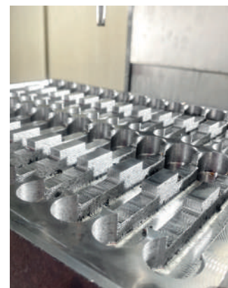
Interrupted Pocket milling operation
