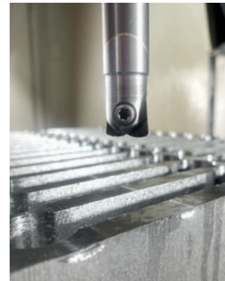
Helical Interpolation and slotting operations
