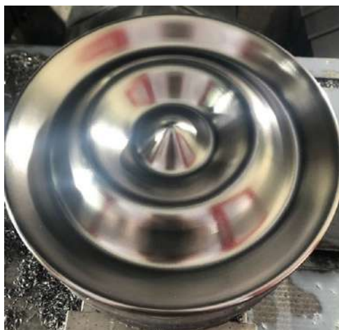
Surface finishing with more challenging cutting conditions
