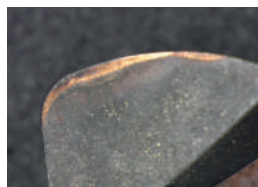
Flank and Rake wear after 67 min
